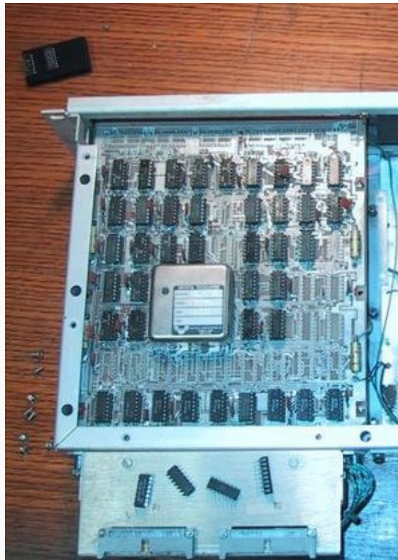
A real-time clock built of TTL chips around 1979.
